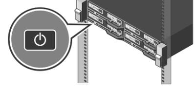
**🔍 NOTE:** Ensure that the enclosure is powered on before turning on the sled(s).
